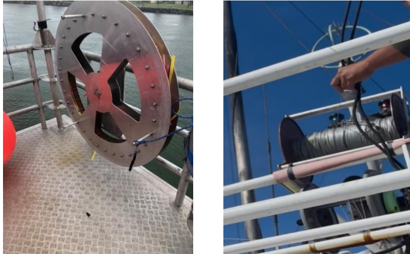
Figure 3.11 Engineered tori line storage systems used within the ETBF, illustrating alternative approaches to storing and deploying tori lines. Improved storage systems reduce tangling, enhance deployment efficiency and support safer handling during fishing operations.
