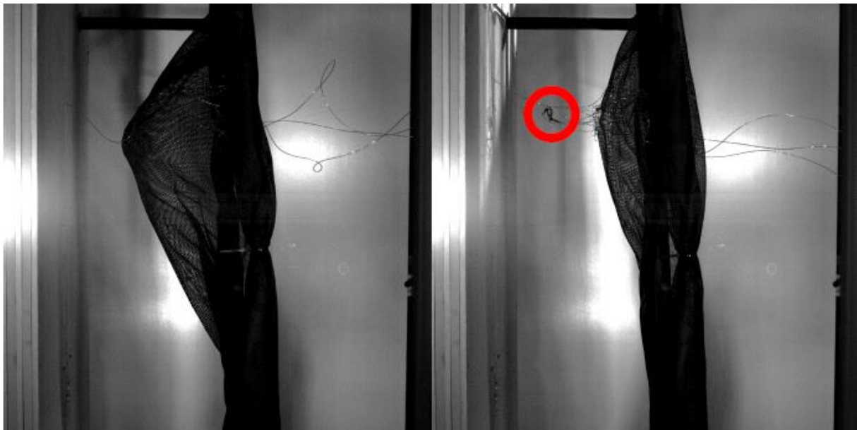
Figure 3.14 Flyback simulation testing of safety screen configurations under controlled conditions, comparing slack and taut screen tension. The slack configuration captured the weighted swivel, while the taut configuration failed under impact loading (circled in red).
