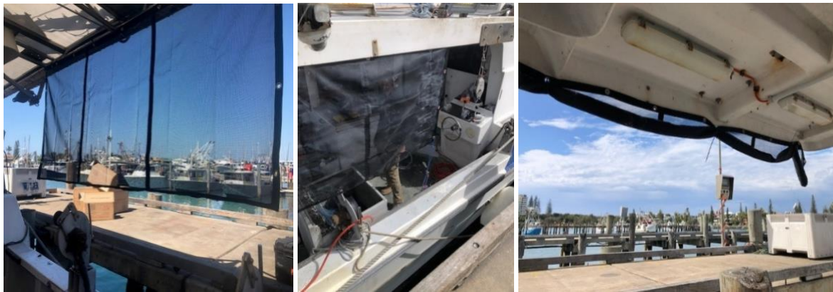
Figure 2.13 Installed flyback safety screens on commercial fishing vessels, demonstrating visibility, coverage of working areas and retractable design for operational use.
