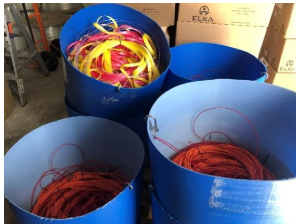
Figure 2.3 Common industry method for storing tori lines using modified 200l plastic drums, illustrating typical storage practices and associated handling considerations.
