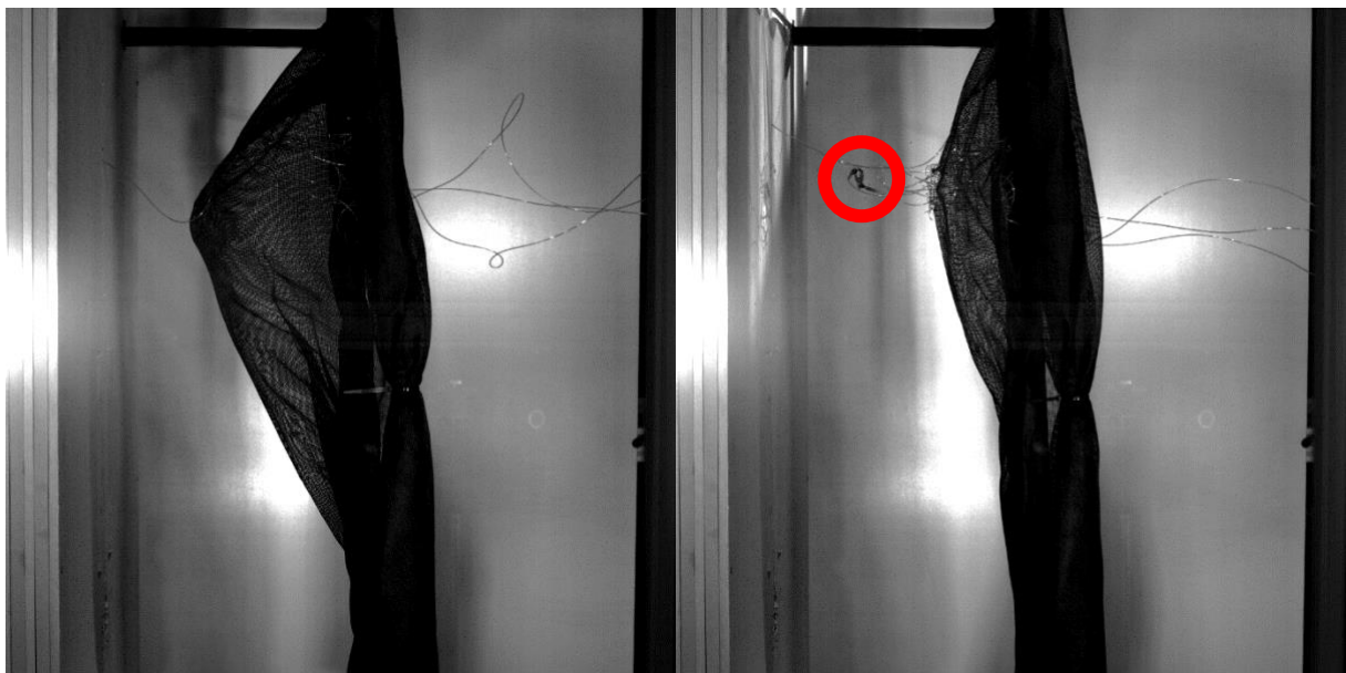
Figure 15: Demonstration of a no punch through (left) and punch through, highlighted in red, (right) of the protective screen
