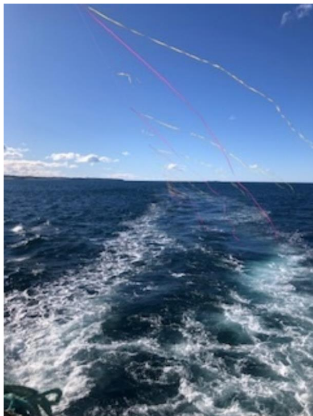
Figure 2.1 Photograph of a deployed tori line astern of a tuna longline vessel in the ETBF during line setting, illustrating typical configuration and aerial extent under operational conditions.
