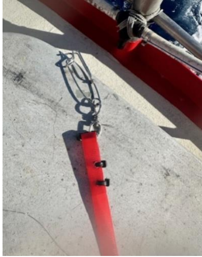
Figure 3.10 Single strand pallet strapping fixed in place with zip ties, attached to stainless steel ring and shark clip for ease of attaching.
