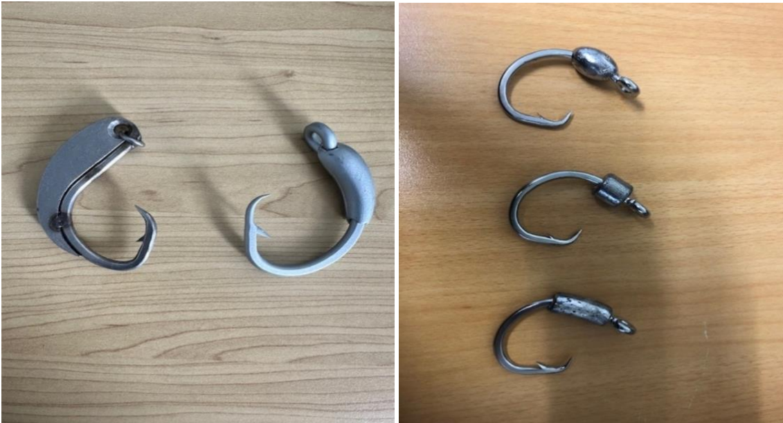
Figure 1 Procella original and improved version (left) and prototype weighted hooks (right) showing decreased hook gape due to positioning of weight. Procella variants were tested in flyback simulations.
