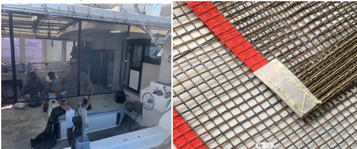
Figure 5: Mock up of flyback safety screen and Kevlar reinforced fiberglass screening
