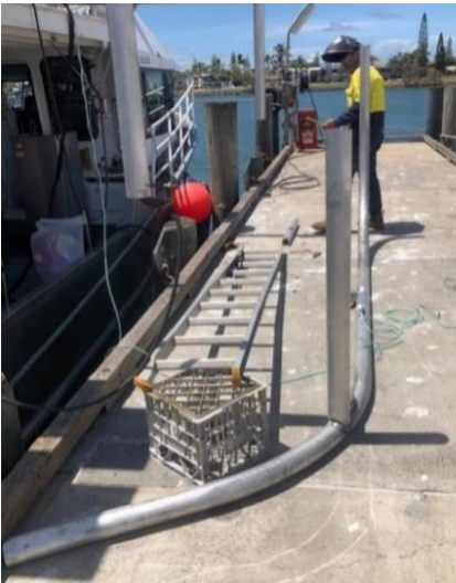
Figure 11 Images of the construction of the flyback bar on the FV Scorpion.
