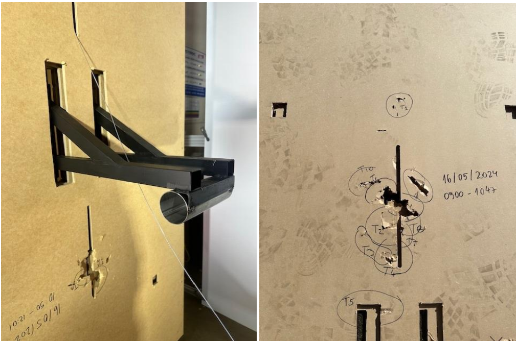
Figure 13 Close up of the testing of the diameter of the flyback bar and the damage caused from simulated flyback events.
