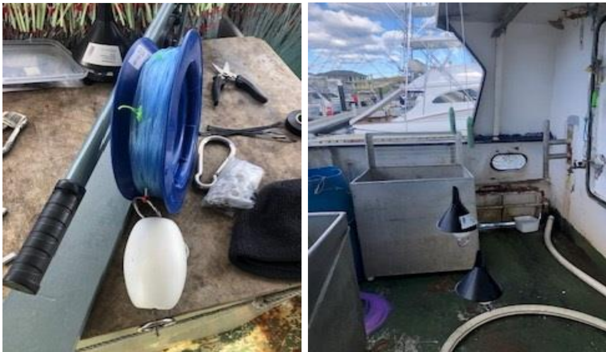
Picture 1: Tori line extent measuring device and fabricated drogue attachments
